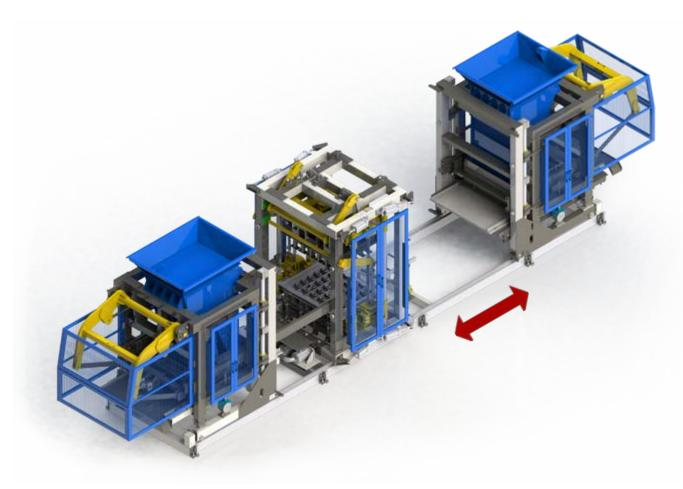
Heavy-duty welded machine frame is equipped with electric motor driven height and length adjustment devices. Both base and face concrete filling systems are connected to the machine's moulding unit via hydraulic clamps. This system reduces time and effort during mould change and maintenance works.
