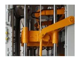
Mould and compaction head carriers are mounted on four chrome-plated guiding columns. These columns are supported by linear bearings, which stabilize the whole structure during production cycle. The mould is attached to the mould carrier via 4 airbags. The compaction head is fastened to the compaction head
