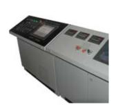
Production process is controlled by one operator via control panel equipped with a LCD touchscreen, which displays all parts of the system in individual pictures. Upon touching the chosen unit the menu appears showing current operating mode and preset parameters. The parameters can be changed in real-time without stopping the production. The software has user-friendly interface while all information is written in customer's preferred language.
